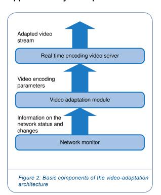
The designed video-adaptation solution (Figure 2) [3][4] consists of three components: a network monitoring tool, a video-adaptation module and a real-time encoding video server. The network-monitoring tool observes traffic flows in the network and gives this information to the adaptation module. The adaptation module chooses video-encoding parameters according the transient network status; the video server encodes and transmits the resulting video stream.
