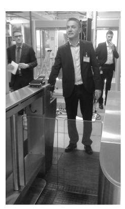
Fly solution, Morphowave, a fingerprint controller product generated within the project by Safran Identity & Security SAS and an example of how innovation speeds up security. By simplifying deployment and improving user experience, advanced biometrics facilitate security for agents and users; swiping four fingers across a scanner
