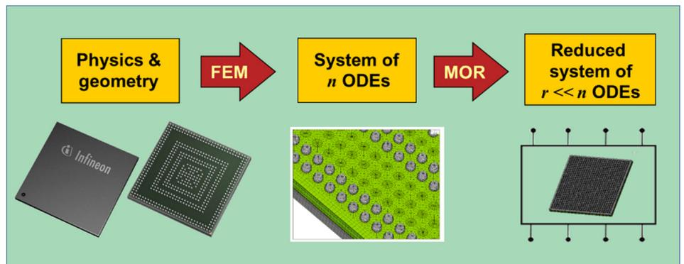
Model order reduction allows an automatic transition from a large-scale finite element model consisting of millions of ordinary differential equations (ODE) into lower order highly accurate surrogate.
