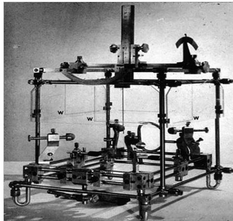
Figure 6.2- Stereotactic frame designed by Horsley and Clark used for neurosurgical practices. *Courtesy of Neupsy Key*<sup>6.2</sup>
