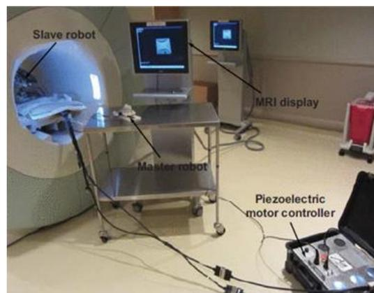
Figure 6.8 - Source-replica teleoperated MRI guided system based on Piezoelectric motors for needle insertion [90]
