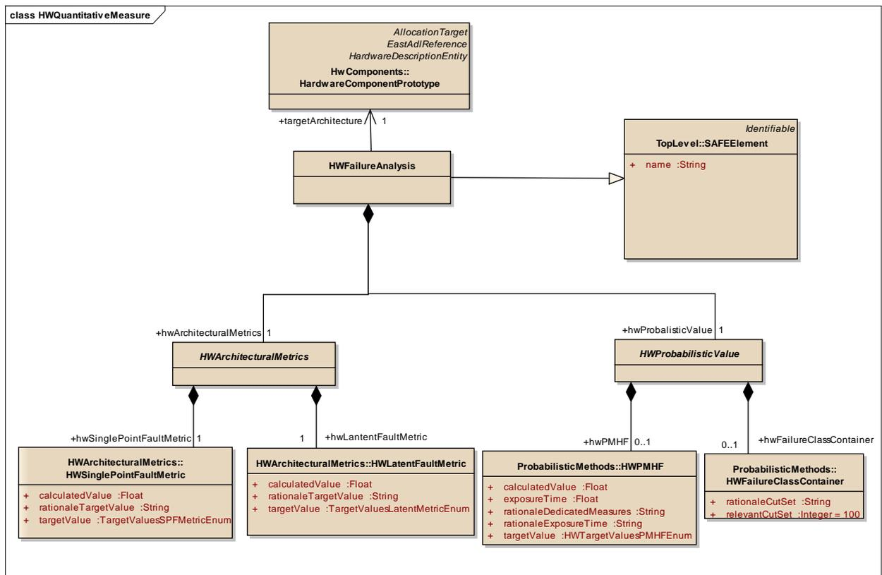
Figure 6: HWQuantitativeMeasure - (Class diagram)
