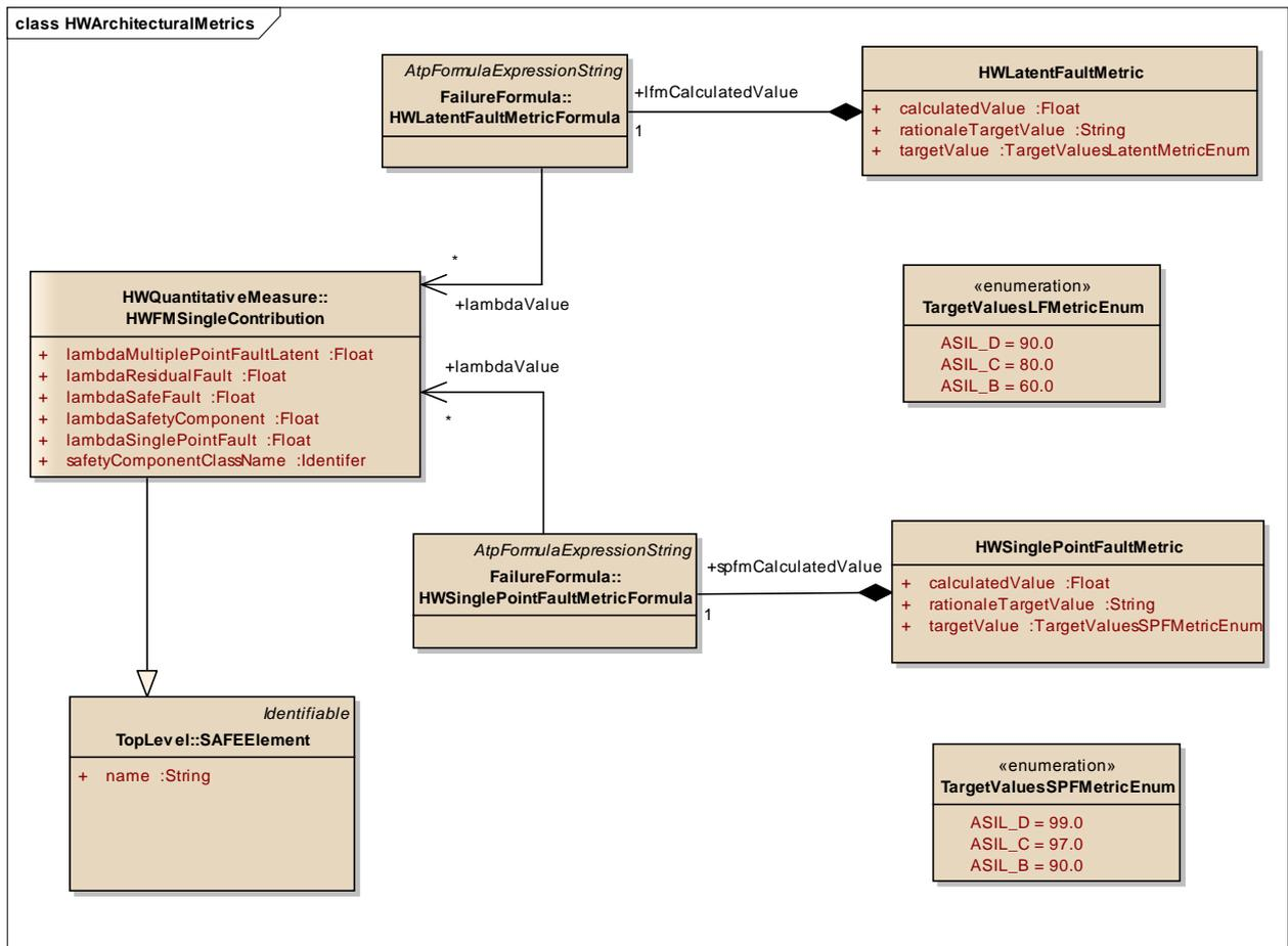
Figure 8: **HWArchitecturalMetrics** - (Class diagram)
