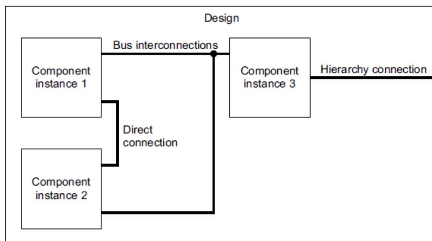
Figure 16: Design representation in IP-XACT
