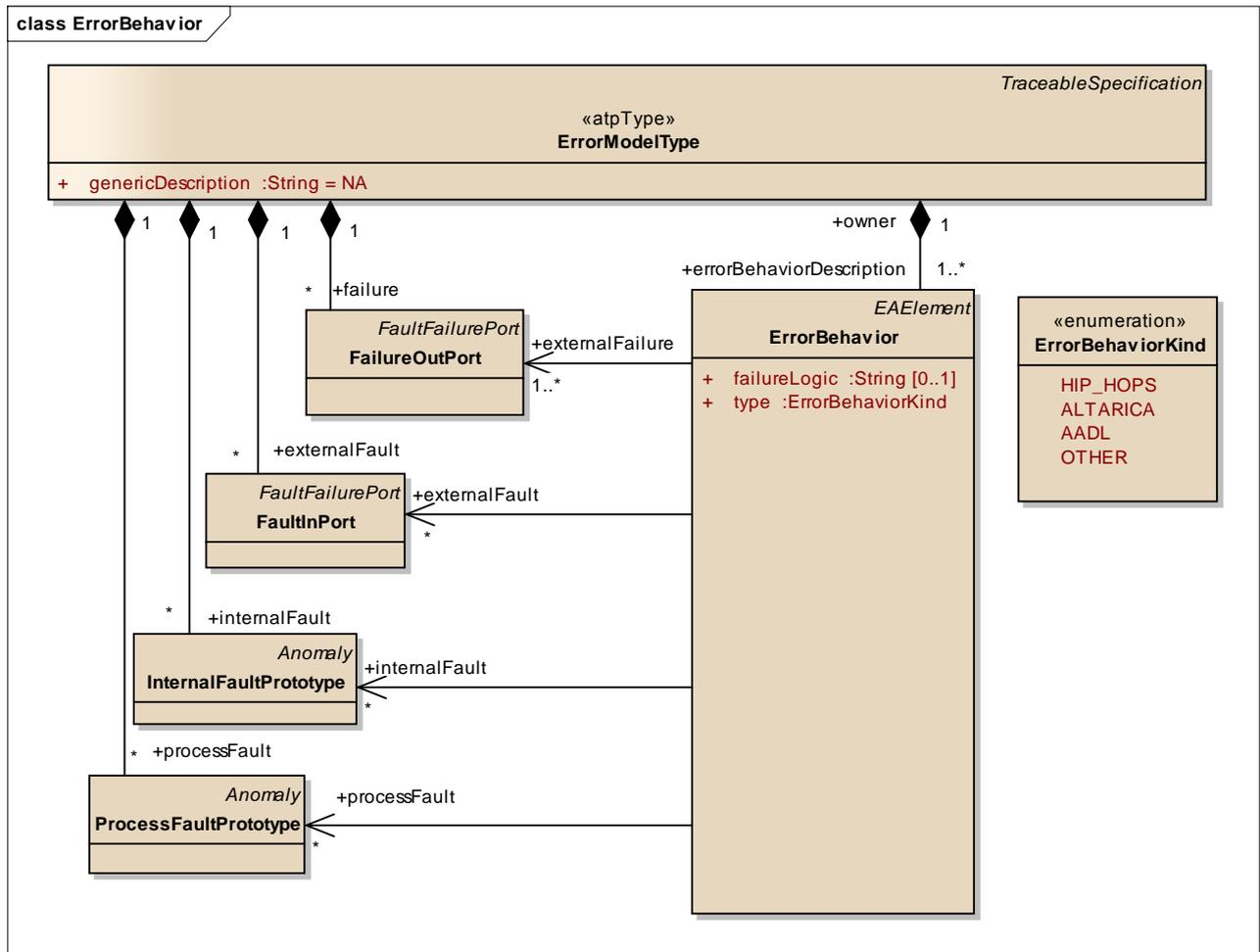
Figure 9: Class diagram for Error Behavior in the EAST-ADL2 Dependability
