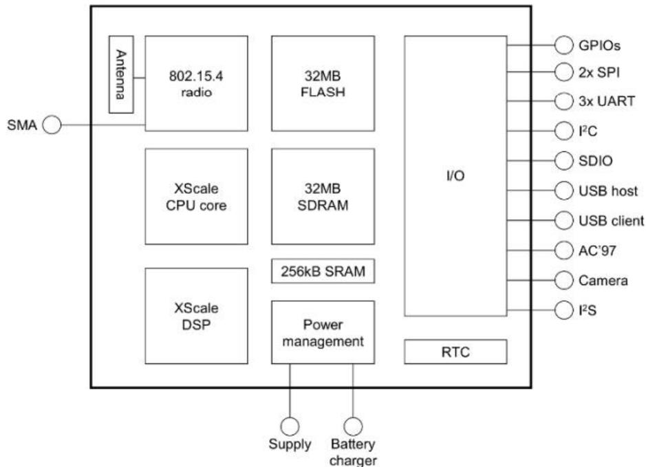
Figure 43: Block diagram of embedded computer Imote2
