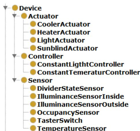
Figure 31: Example Classification of Building Equipment
