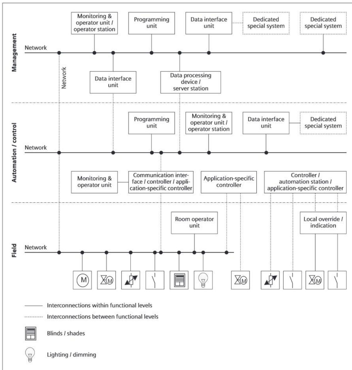
Figure 3: Possible interconnections in three-level functional hierarchy
