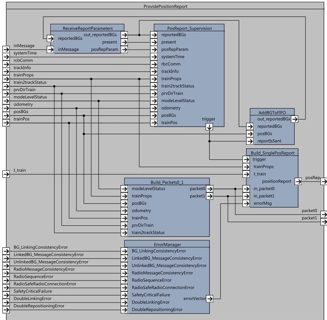
Figure 25. Provide\_Position\_Report component SysML diagram
