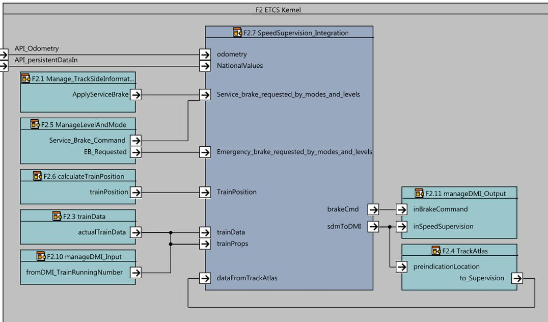
Figure 10. F2: ETCS Kernel SysML diagram with focus on F2.7 SpeedSupervision\_Integration component.
