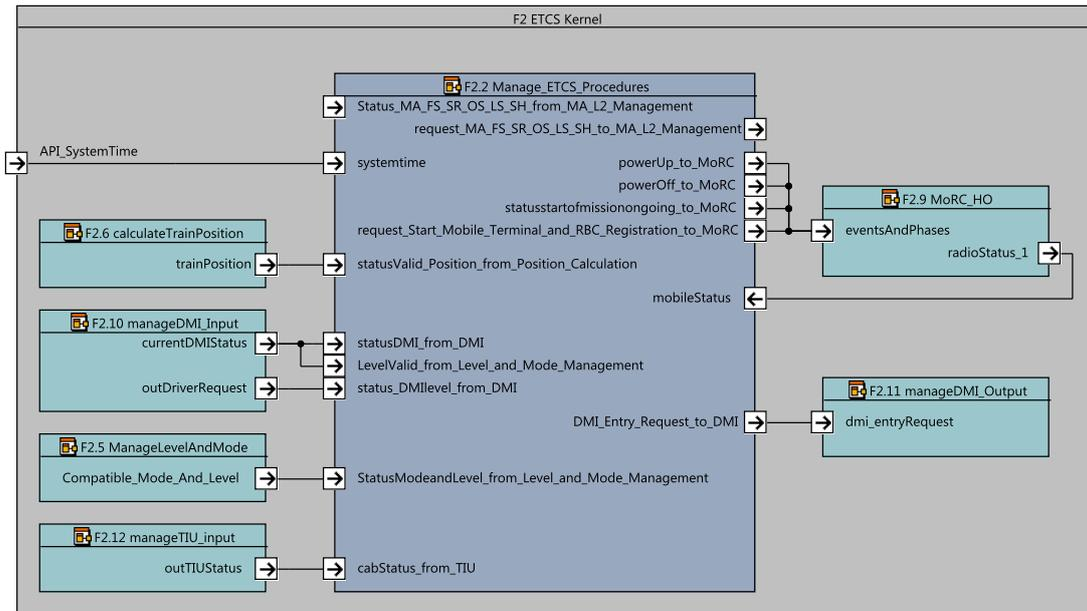
Figure 5. F2: ETCS Kernel SysML diagram with focus on F2.2 Manage\_ETCS\_Procedures component.
