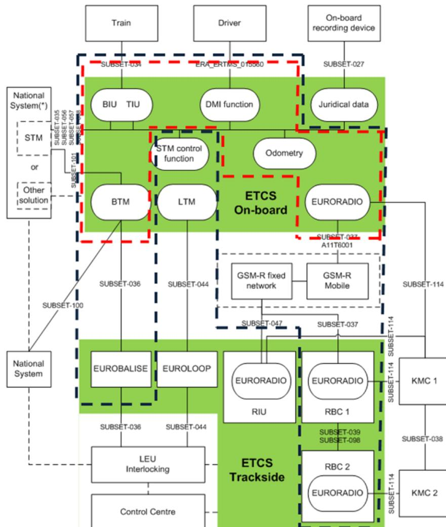
Figure 1. Scope of openETCS OBU model system according to ERA TSI Chapter 2.5. Functional blocks in the scope of openETCS have been marked by the dashed black line. The dashed red line shows the OBU blocks in the scope of openETCS.
