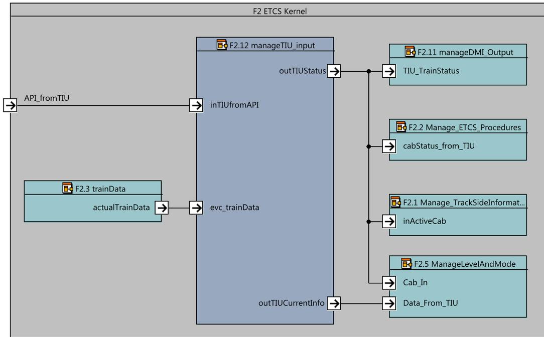
Figure 15. F2: ETCS Kernel SysML diagram with focus on F2.12 ManageTIUInput component.
