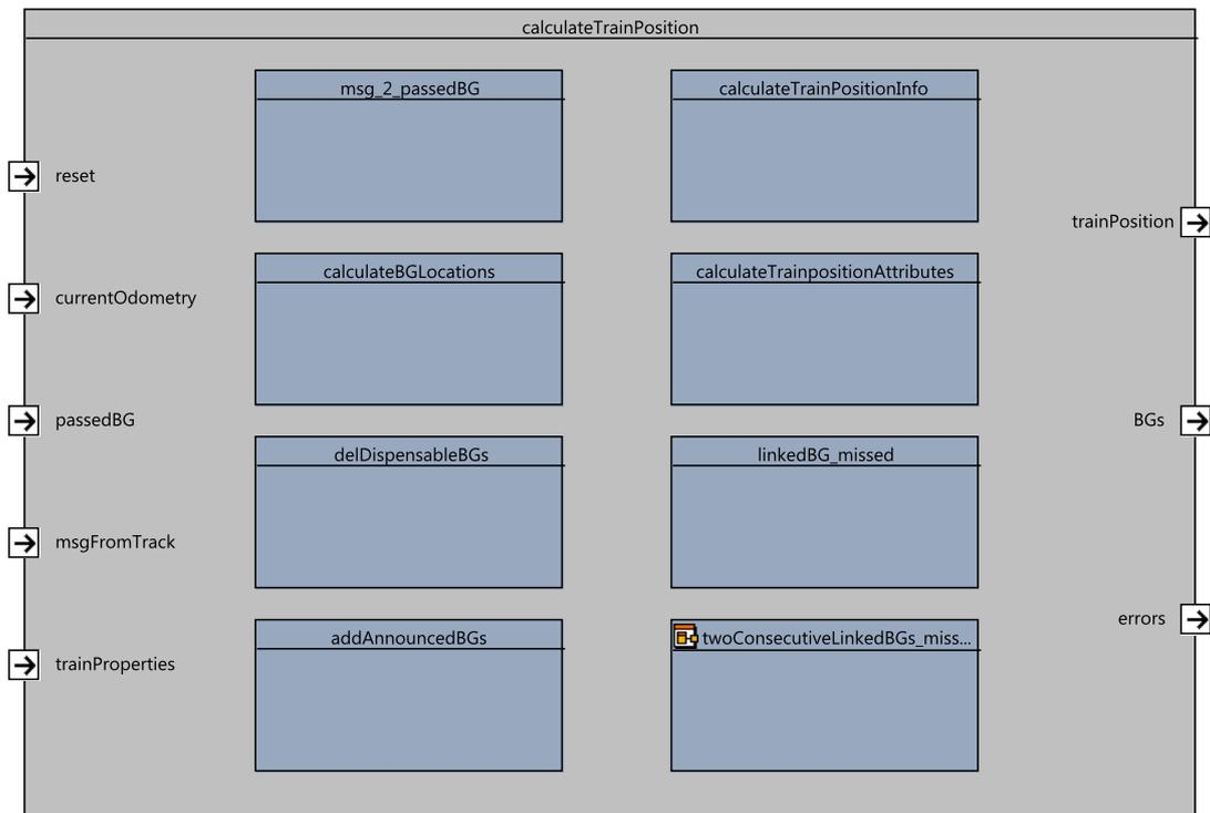
Figure 23. calculateTrainPosition component SysML diagram.
