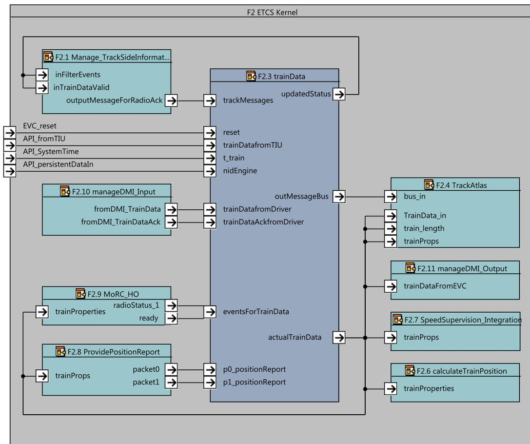
Figure 6. F2: ETCS Kernel SysML diagram with focus on F2.3 trainData component.
