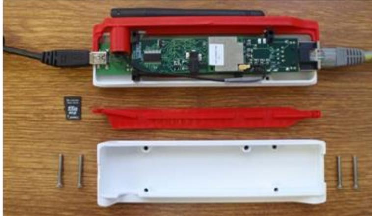
Figure 52: Uncovered firewall prototype microcomputer-based on Gumstix Verdex developed at Masaryk University
