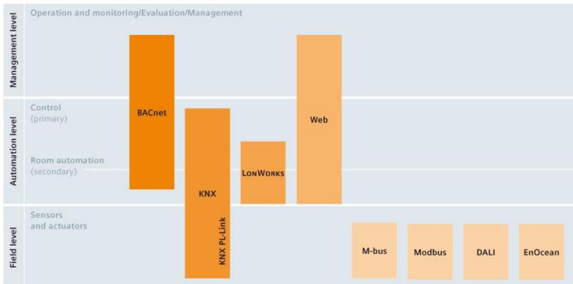
Figure 6: Communications protocols as used in the different levels of the automation pyramid [10]
