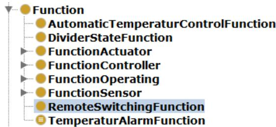
Figure 35: Example Automation Functions
