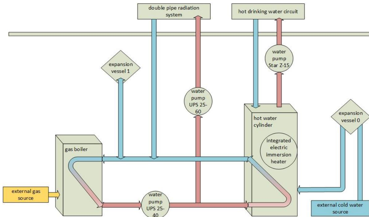
Figure 4-10: Overview of a Heating Circuit.
