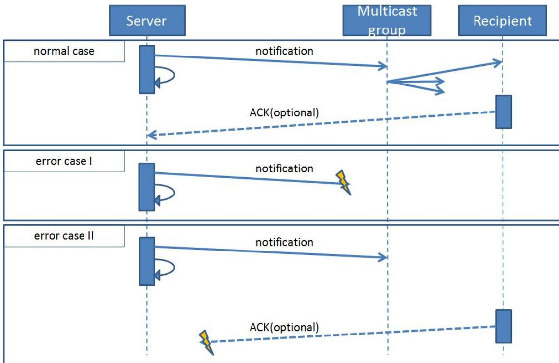
Figure 4-23: CPAT-05: Asynchronous Announcement to a Group of Receivers (1)
