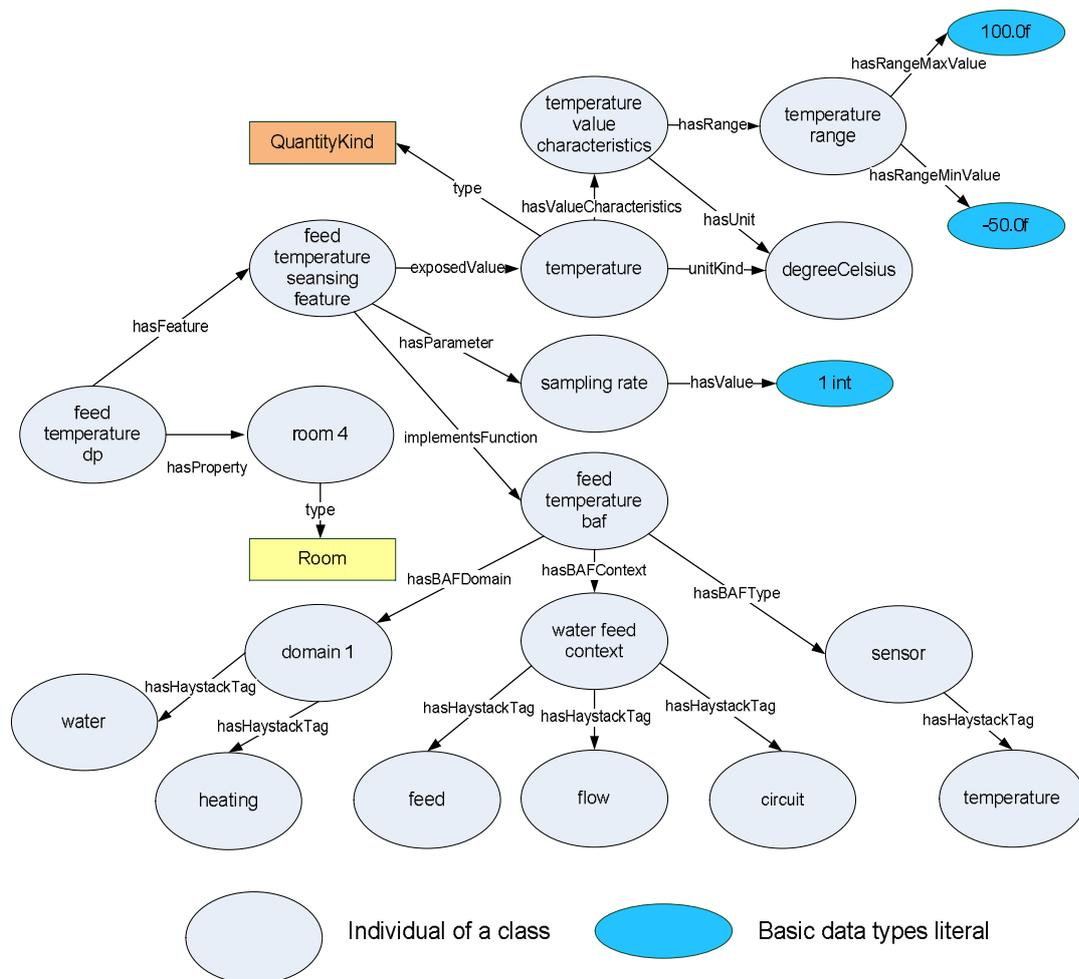
Figure 4-14: Ontology Example: A Feed Temperature Data Point
