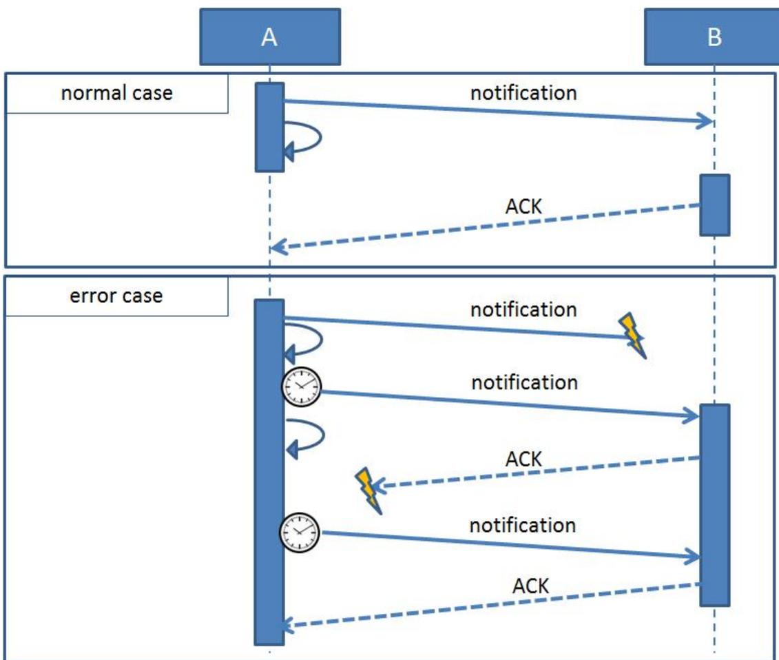
Figure 4-21: CPAT-03: Asynchronous Request Response
