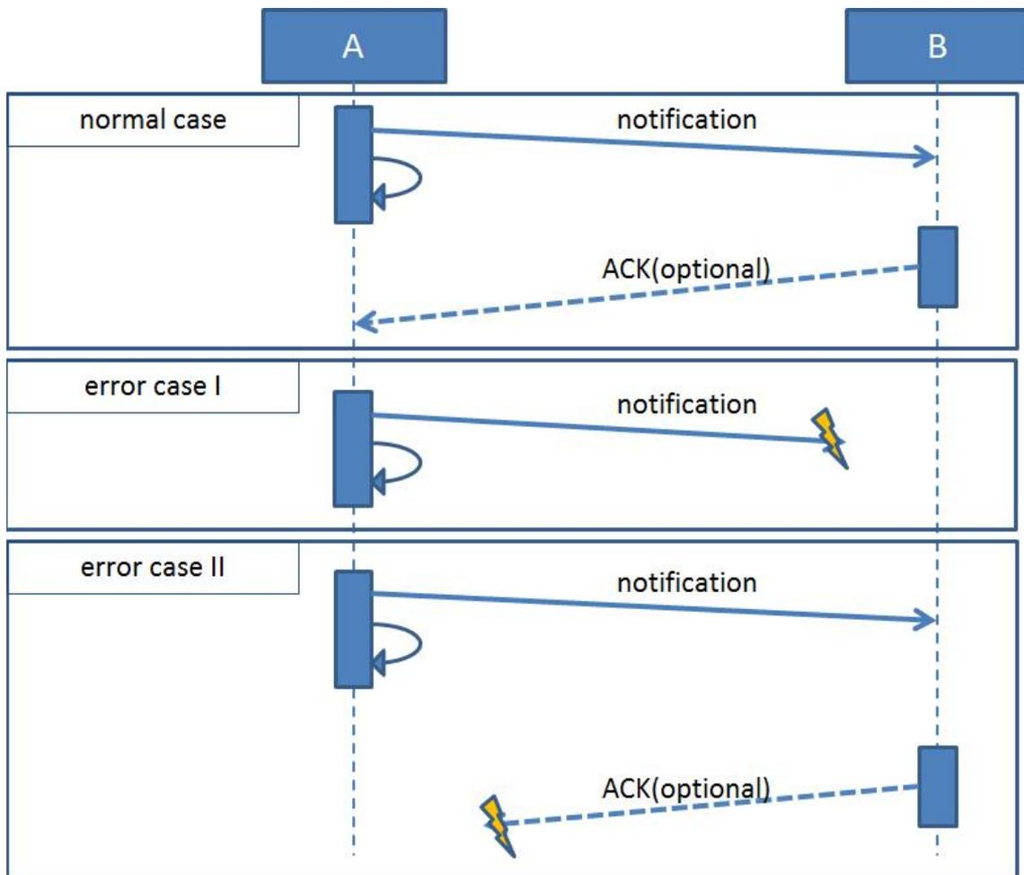
Figure 4-22: CPAT-04: Asynchronous Notification
