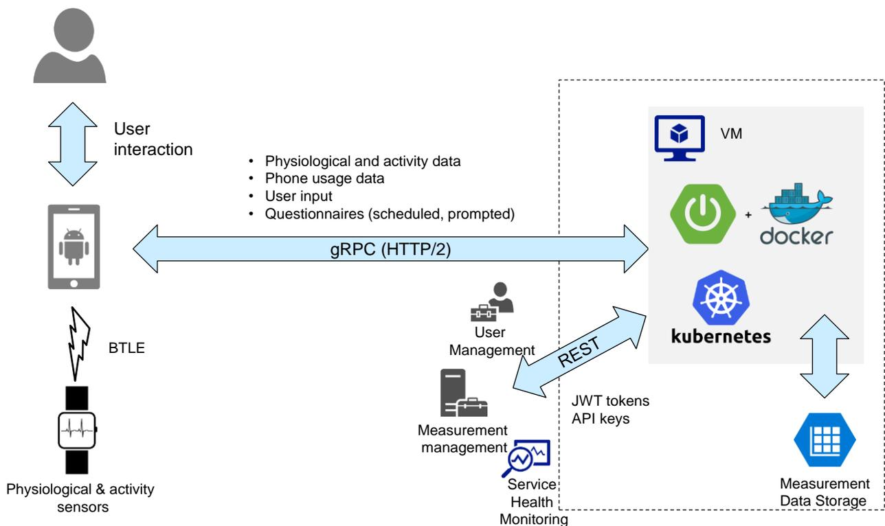
Figure 28. The overall scheme for physiological and activity data collection in the Finnish pilot.
