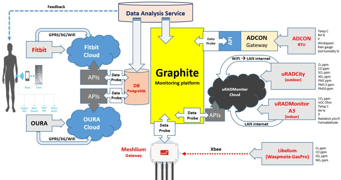
Figure 4. Sensors Architecture.
