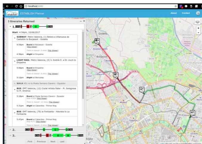
*Figure 11. Example of a multimodal routing, which combines a leg by train, another walking and a final leg by bus.*
