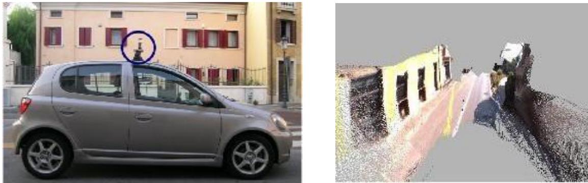
Figure 34: Vehicle with camera (left); Dense 3D reconstruction (right)
