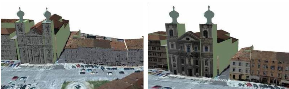
Figure 37: Terrestrial laser scans of the building facades (left) and terrestrial ortho-photos wrapped on the facades (right)
