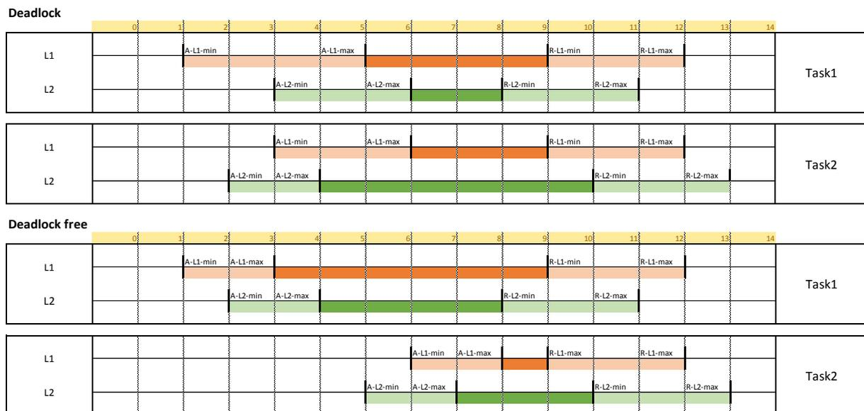
Figure 29: Two scenarios with interleavings between two tasks
