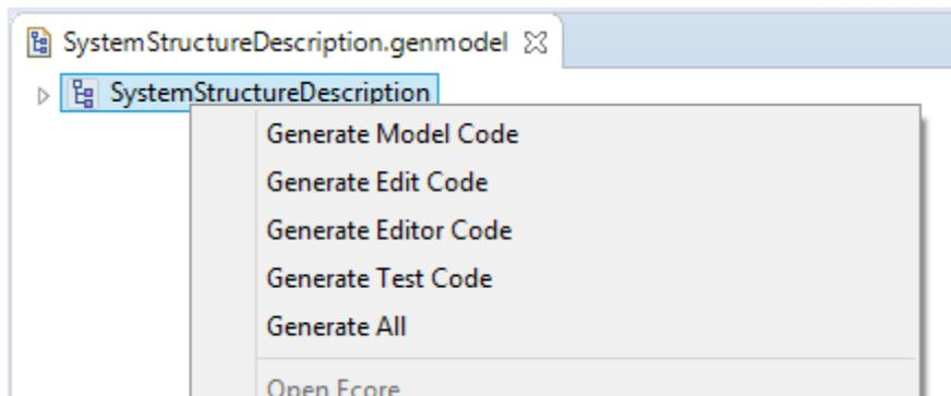
Figure 7. Generating model code
