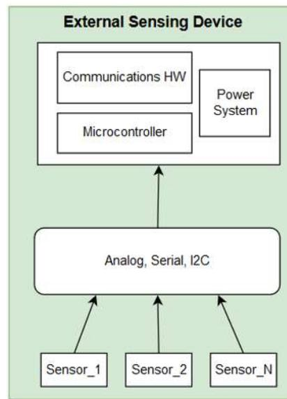
**Figure 51: High level ESD component diagram**
