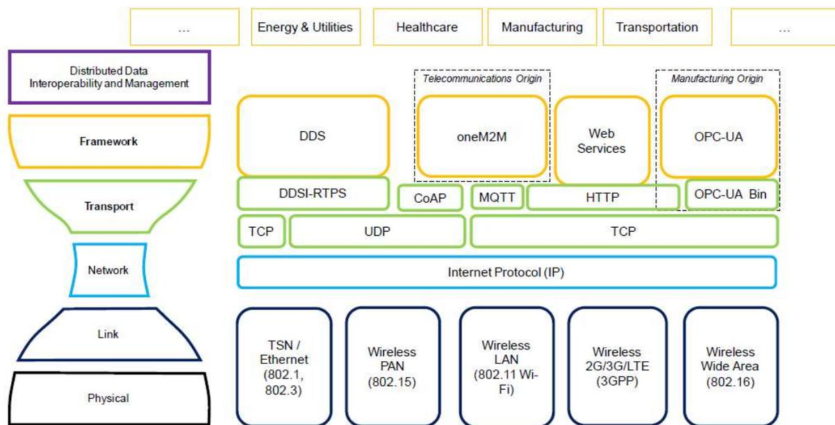
Figure 26: DDS and other Protocols in the Network Stack [27]
