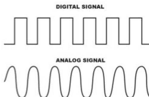
**Figure 35: Digital and analog signal waves**
