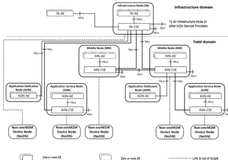
Figure 19: Configuration supported by oneM2M architecture.
