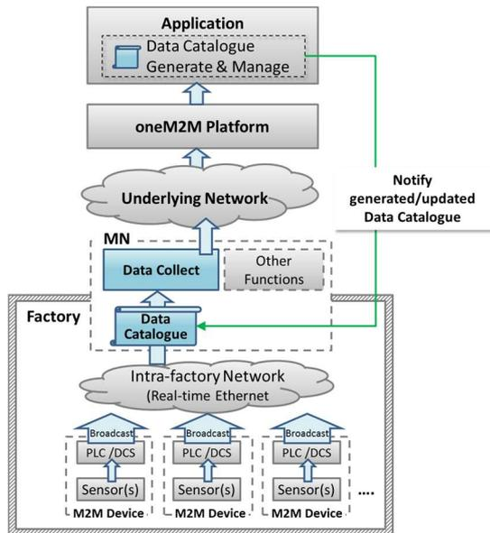
**Figure 22: High-level Illustration of On-demand Data Collection for Factories**
