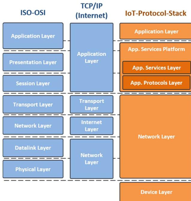
**Figure 2: Representation of the IoT-protocol-stack and comparison with the ISO-OSI-model as well as with the consolidated TCP/IP (Internet) one.**
