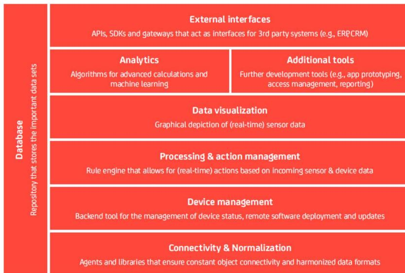
**Figure 16: The eight major building blocks of an IoT platform [16]**
