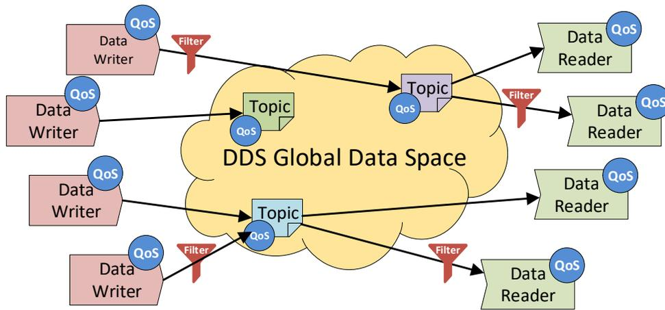
Figure 25: DDS Global Data Space Concept, derived from portals.omg.org
