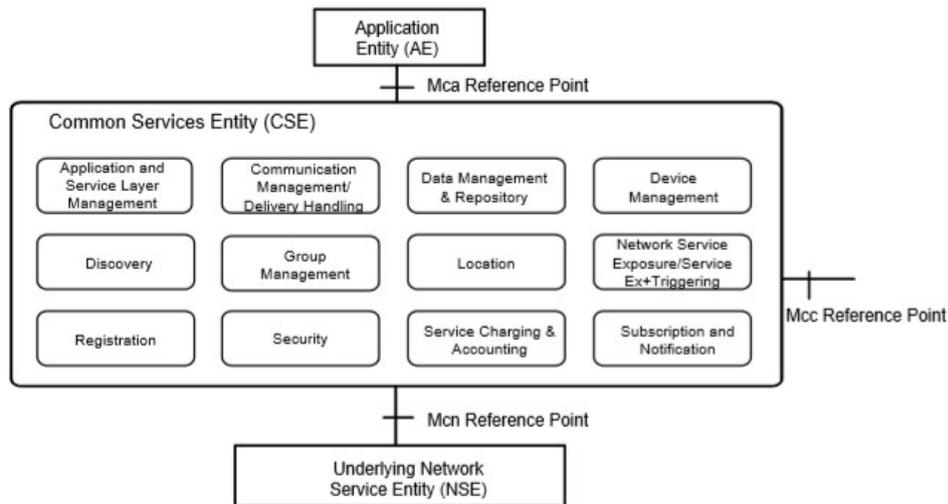
**Figure 20: Common Service Function (CSF)**
