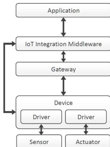
**Figure 3: IoT Reference Architecture [12]**
