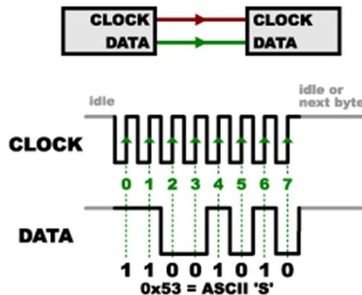
Figure 37: Diagram of data communication synchronized by a clock line
