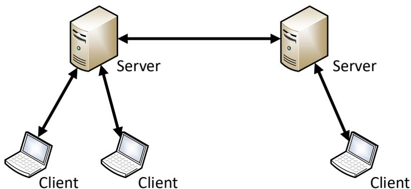
**Figure 31: Distributed Architecture of XMPP**
