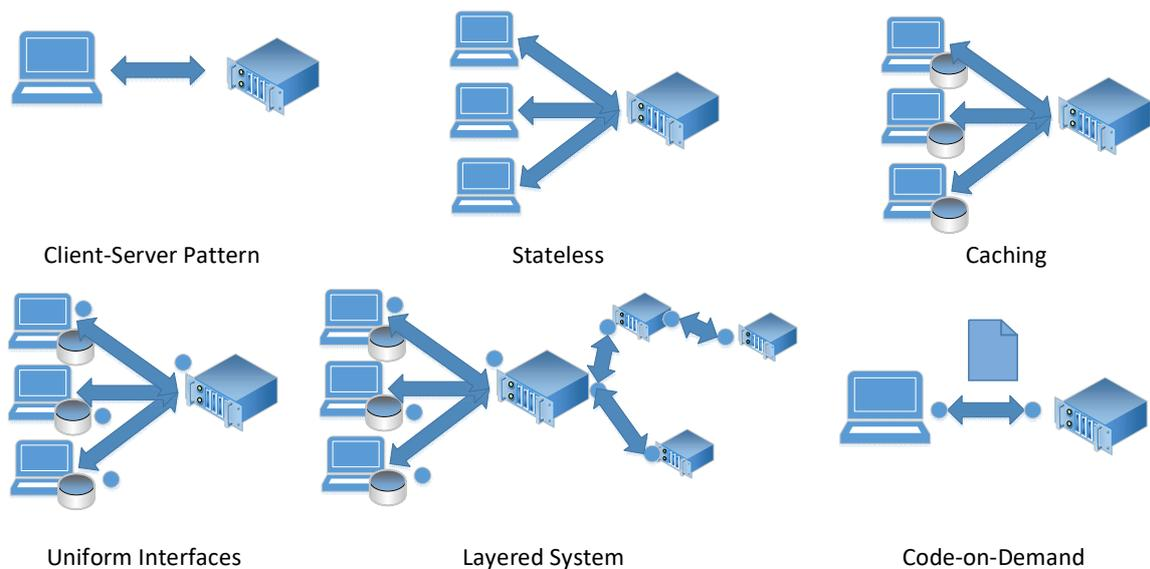
**Figure 29: Features of a RESTful Architecture**
