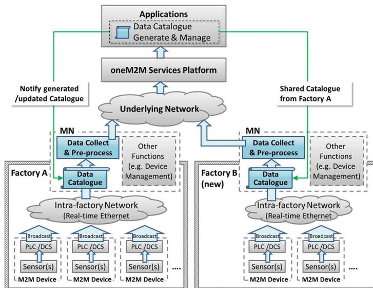
**Figure 23: High-level Illustration of Data Process for Inter-factory Manufacturing**
