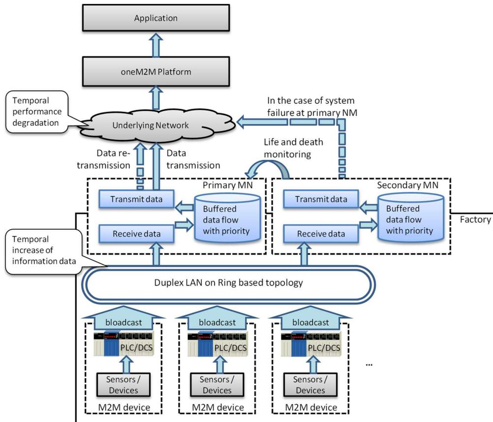
**Figure 24: High-level Illustration of Real Time Data Collection**
