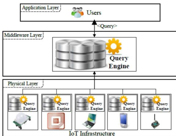
Figure 12: General design model for database-oriented middleware [9]
