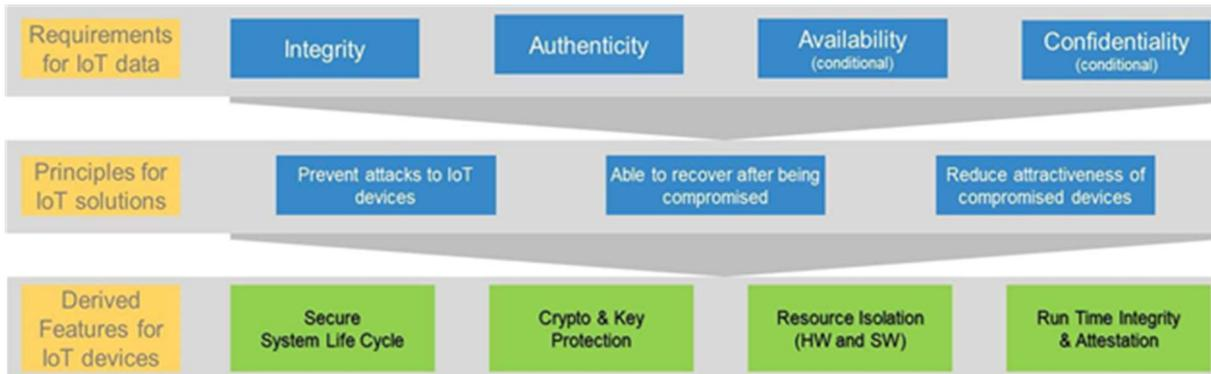
**Figure 40: IIoT device features derived from for IIoT data requirements**
