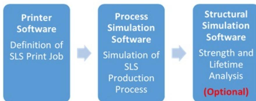
Figure 6.12: Additive Manufacturing - Plastics
