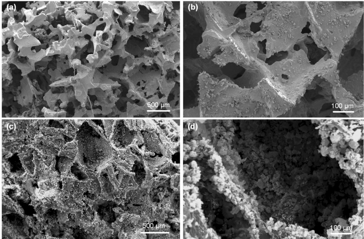
**Figure 2.** SEM micrographs of the PDMS foam before and after MLG loading: (a, b) porous structure of the unloaded PDMS foam at different magnifications; (c, d) MLG loaded PDMS foam at two different magnifications with the pore walls covered with MLG nanoflakes forming a nanomaterial percolation network.
