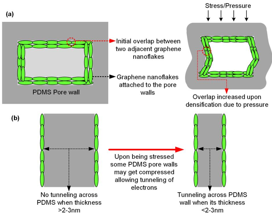
**Figure 3.** Schematic diagram explaining the possible strain induced resistance modulation mechanisms in graphene-PDMS foam sensor: (a) Schematic explaining the conductive domain disconnection mechanism explaining strain induced resistance modulation observed in the sensor; (b) Schematic representation of stress-induced tunneling resistance modulation.
