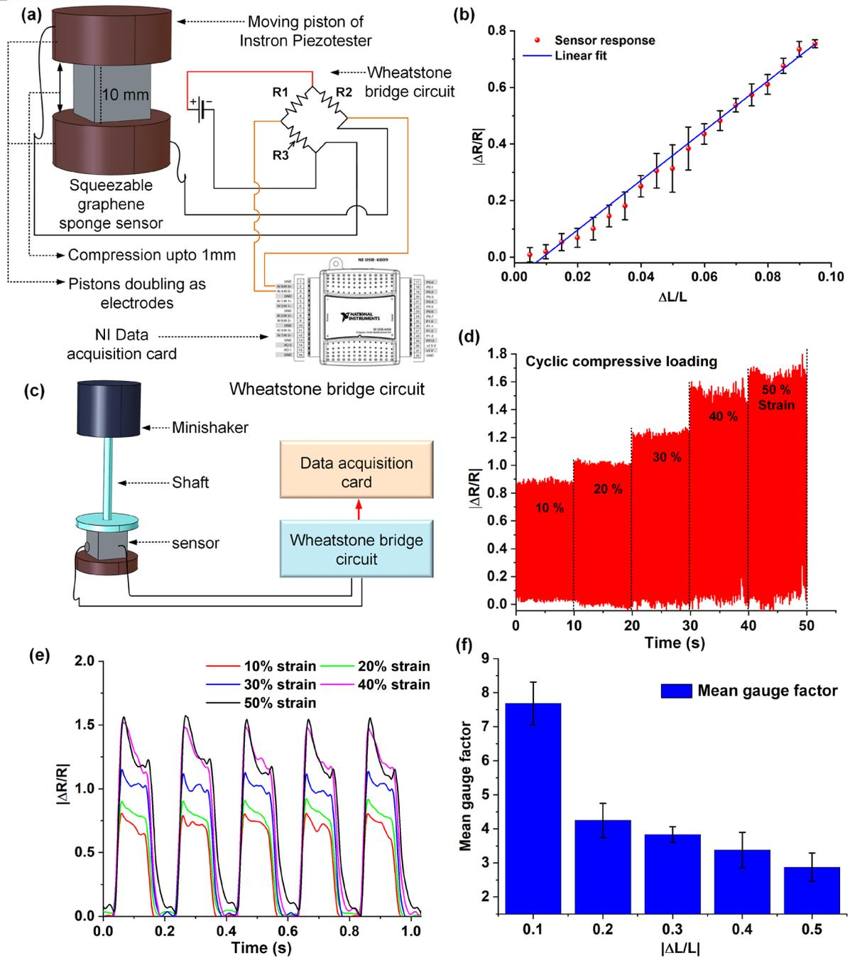
**Figure 4.** Graphene-PDMS foam sensor characterization: (a) Schematic representation of the setup used for conducting the piezoresistivity characterization experiments; (b) Plot of normalized resistance change in the graphene-PDMS foam sensor versus
