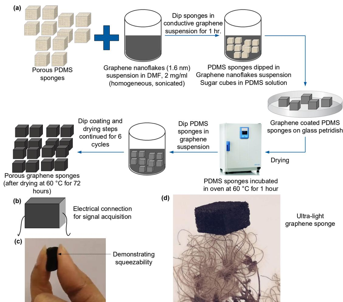
**Figure 1.** Fabrication of the squeezable graphene-PDMS foam sensor: (a) Schematic representation of infiltrating PDMS foam with multilayered graphene nanoflakes (MLG); (b) schematic representation of a single PDMS-MLG foam sensor with electrical contacts; (c) the squeezability and (d) ultra-light nature of the graphene-PDMS foam sensor.
