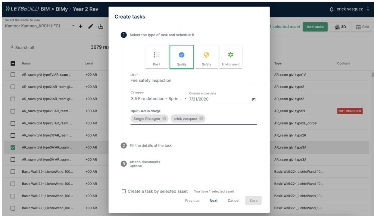
Figure 10: Using LetsBuild BIM module to create inspection tasks linking BIM models, checklists, assignees and more
