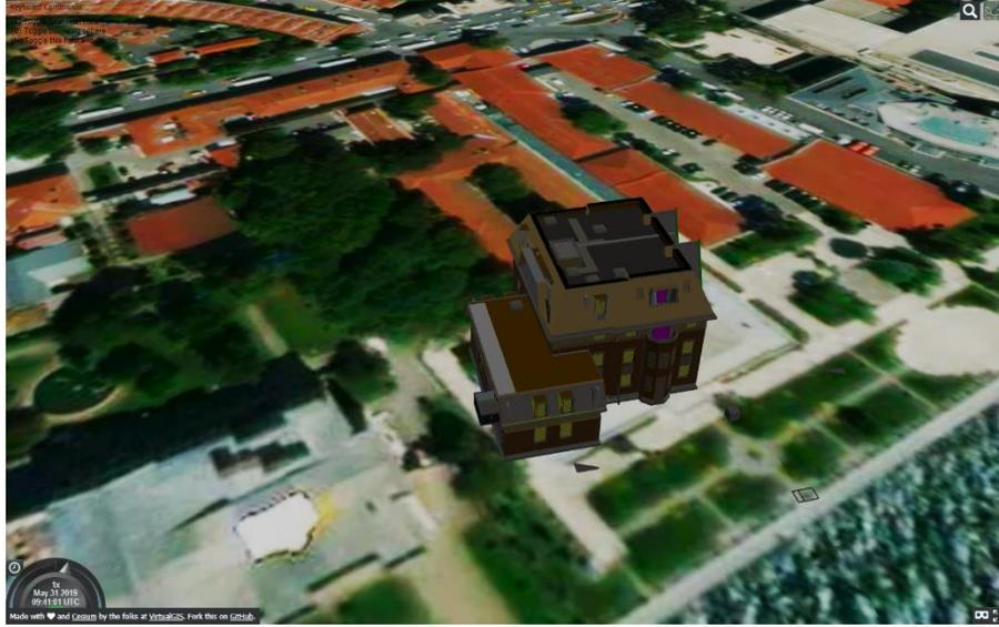
Figure 9: Screenshot on viewing the Schependomlaan BIM model (openBIMstandards, 2015) on a Cesium based web viewer
