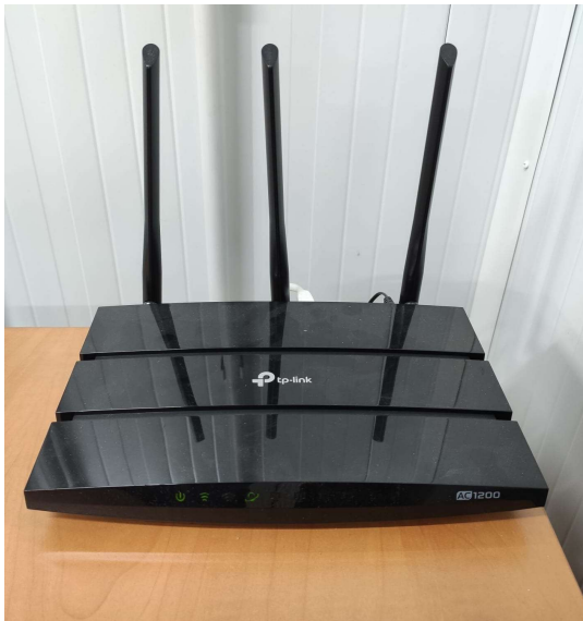
Figure 1: TP-LINK router with 802.11AC and Gigabit Ethernet connectivity
