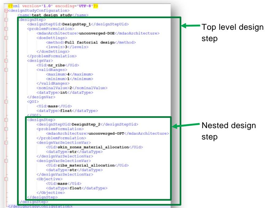
Figure 15: Example of Design Study Configuration file with nested design step
