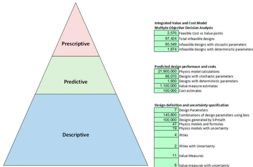
Figure C.3: Set-based design trade-off hierarchy in the UAV design study presented in [33].
