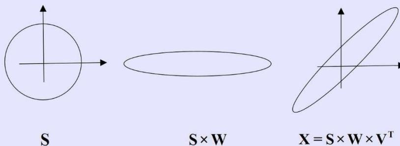
Figure FB5: Visualization of the design or trade-space change and reduction by the application of SVD.
