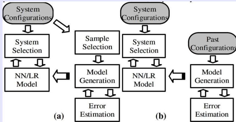
Figure FB3: Overview of DSE using predictive modelling: (a) sampled DSE and (b) chronological predictive models. Source: [26].
