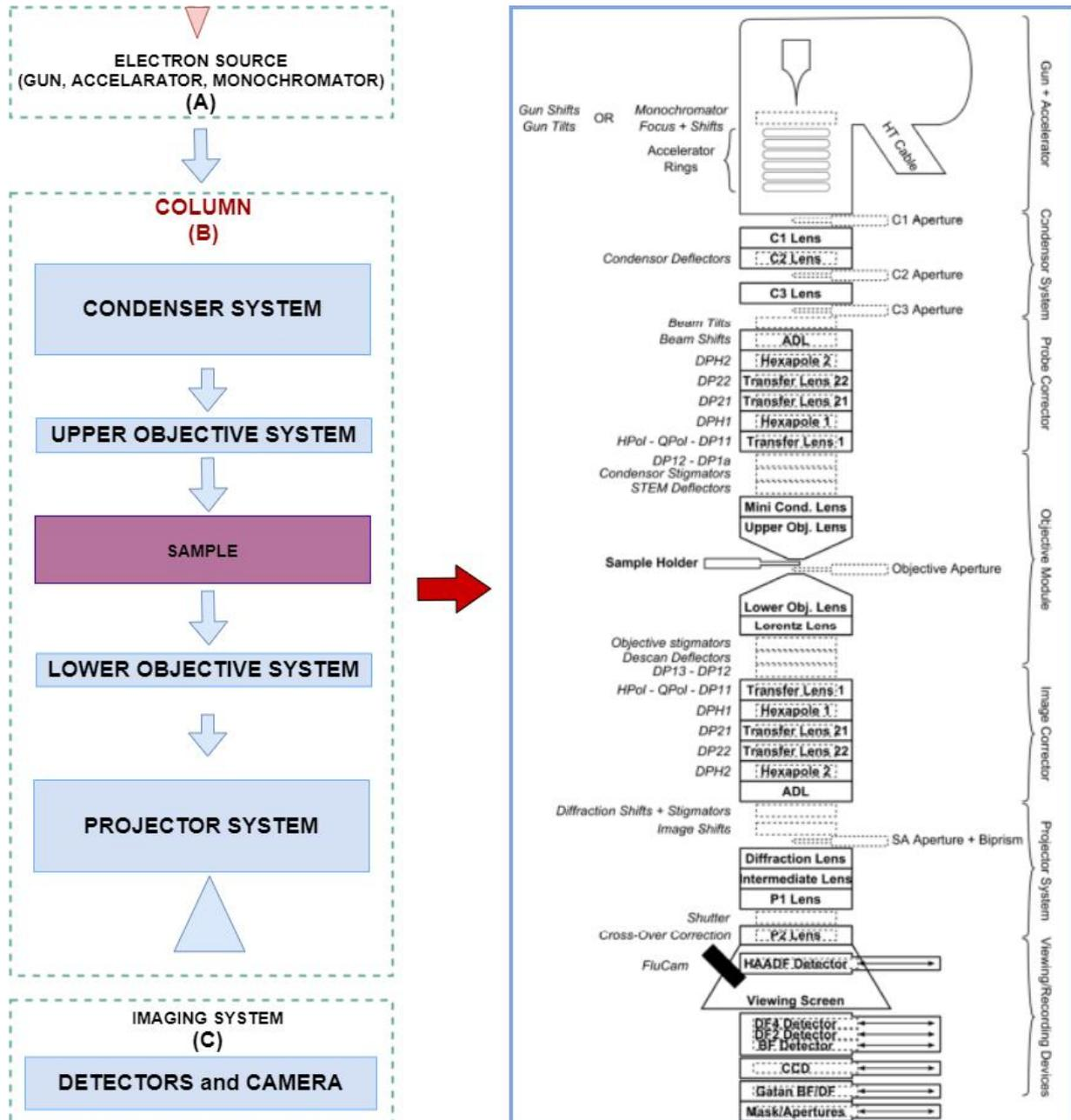
Figure 2: Schematic View of Electron Microscope Components
