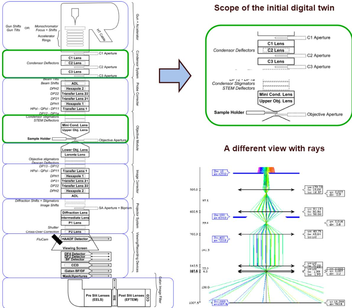
Figure 6 - Electron Microscope Components Included in the Digital Twin
