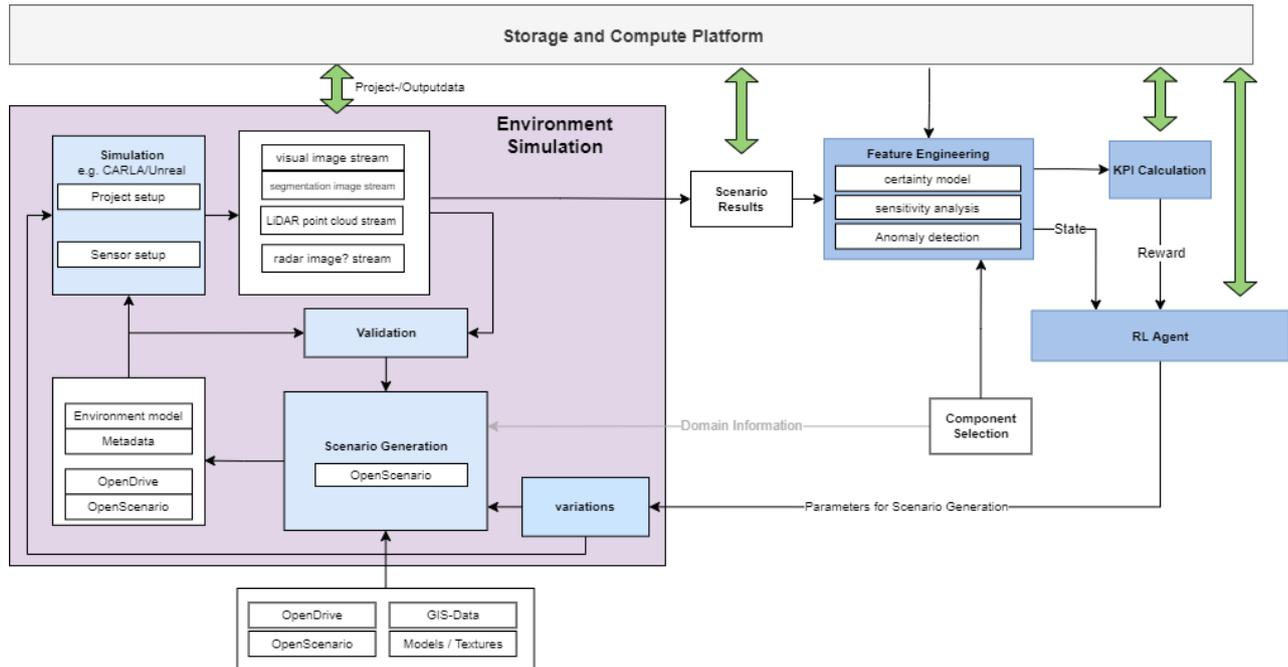
Figure 9 - Process Overview Sub Use Case 1
