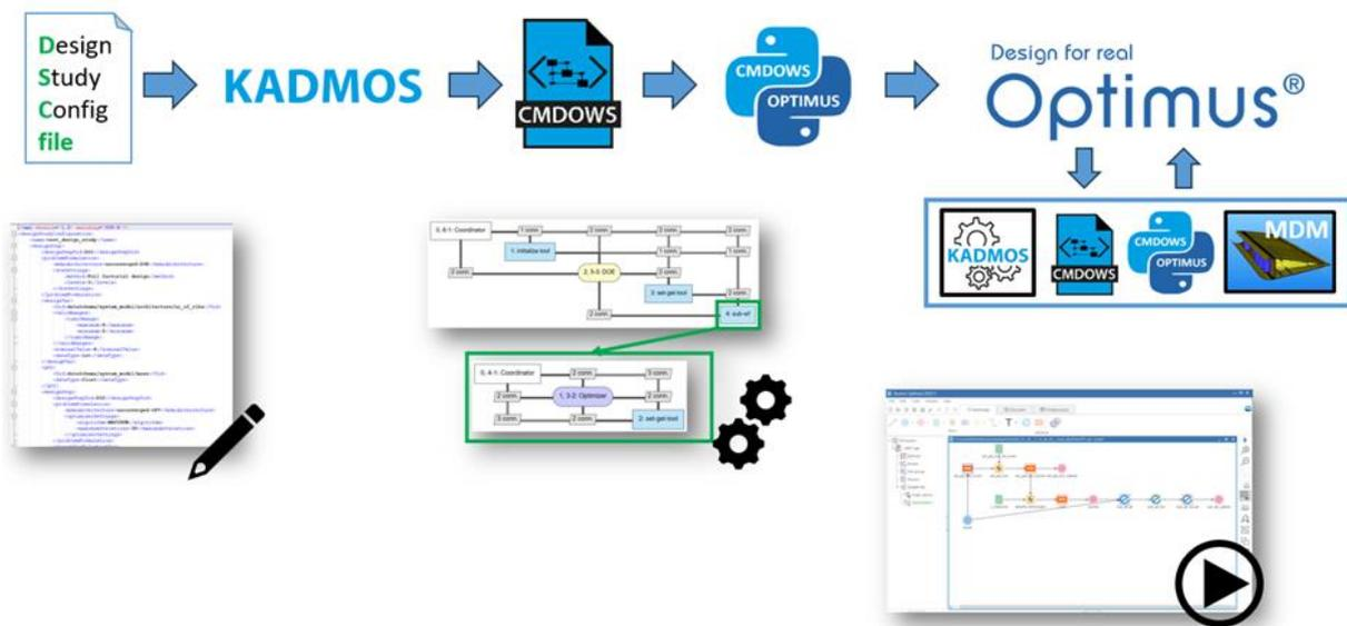
Figure 6: Process of automatically generating a workflow using KADMOS
