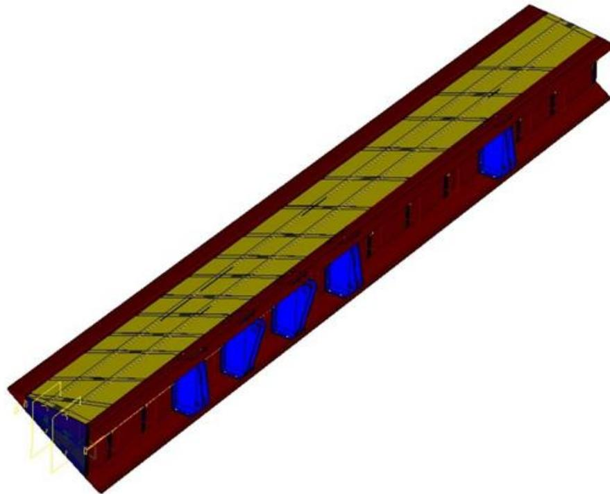
*Figure 3: Aileron design as generated by the MDM application*
