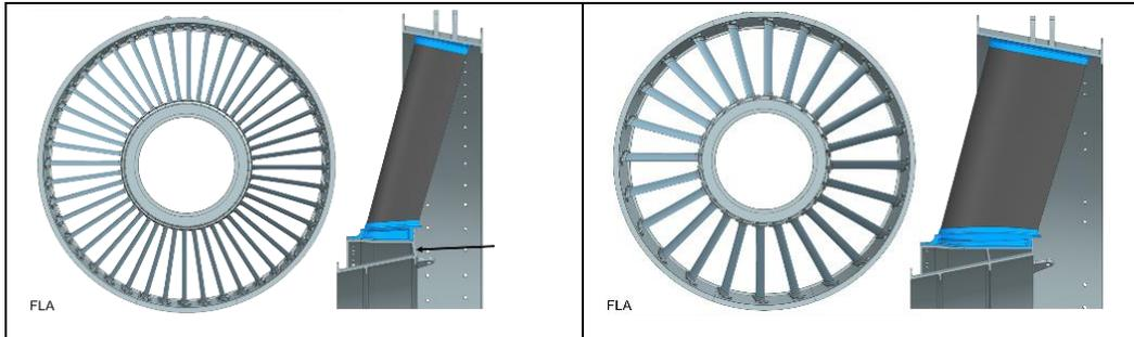
The 16 parameters are included in a DOE for a Design Space Exploration study. The parameters are a mix of continuous real, Nominal discrete and discrete by value, see **Error! Reference source not found.** The distribution used is Latin Hypercube and 132 designs. The number of designs were decided on time available and amount of access to computer cluster.
