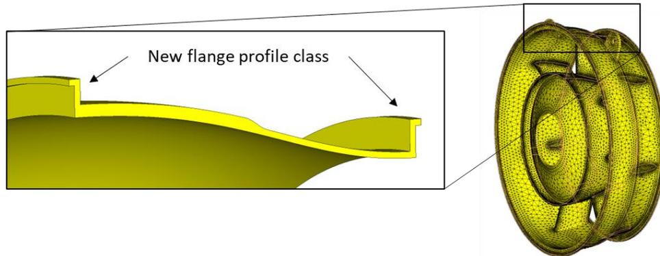
*Figure 14: Cross section of the TRS showing the new geometry of the flange. Right: Complete TRS automatically meshed my using the same KBE functions.*
