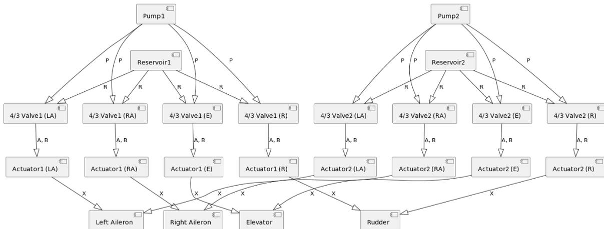
Figure 11: UML diagram (in PlantUMLTM) of an aircraft actuation system with four functions and two circuits, each with a pump and reservoir connected to a valve and actuator for each function.
