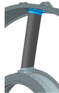
*Parameter:* Vane max thickness, Vane wall thickness, vane hollowness.
