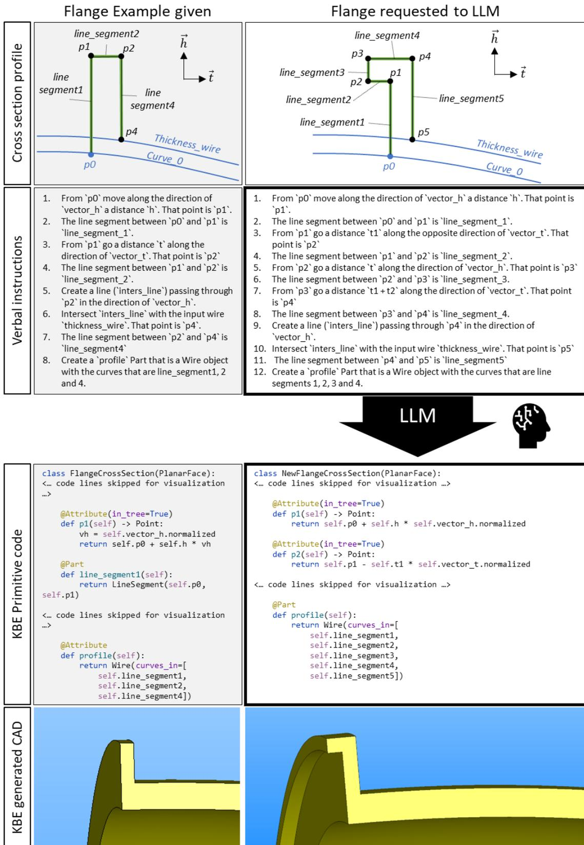
Figure 13: Column comparison between the pre- and post-design change geometry expressed visually and verbally. Prompt and response of the LLM for step 3 are highlighted in the right.
