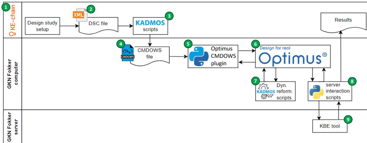
Figure 3: Overview of collaborative architecture optimization design study setup and execution process
