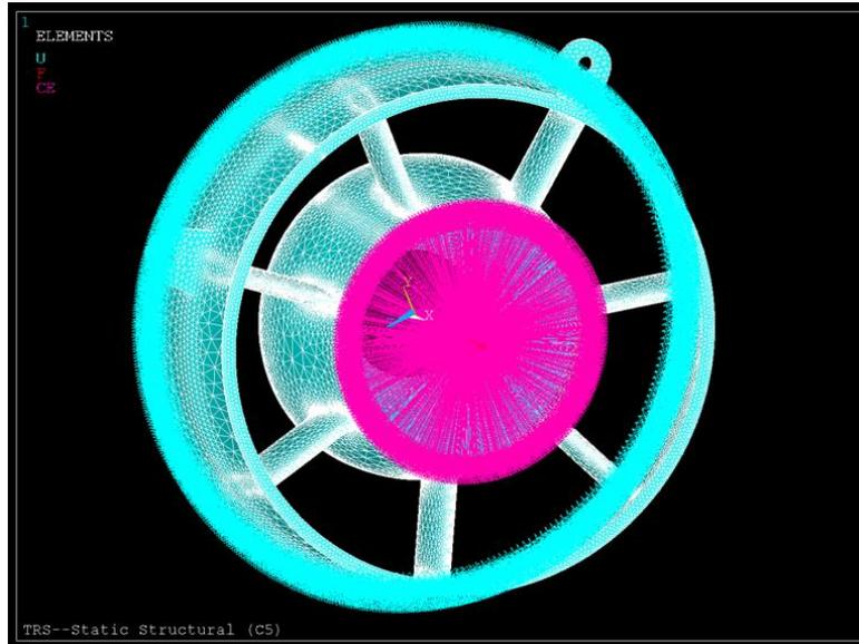
Figure 8: FEM model with loading and boundary condition for a design use case. (view from other side of Figure 6). Screenshot of ANSYS software.
