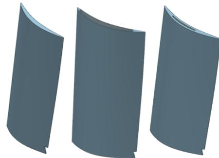
*Parameter:* Outer Case Forward and aft Stiffness Rib Height, Outer Case Thickness.
