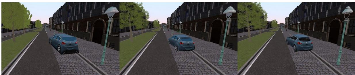
Figure 15 Different level of detail in the environment model (left low, middle medium, right high)
